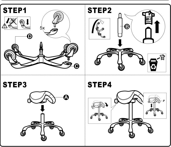
Disassemble Tips: Before you start, you might want to put something down to protect your floor. Turn the stool upside down. Give the seat bottom and hydraulic cylinder protruding end a firm tap with a hammer or a rubber mallet.
